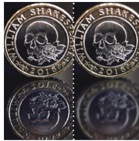
Left - A crisp, sharp reflection is seen in a smooth surface. Right - Very small surface texturing distorts the reflected image causing it to be blurred and indistinct.
