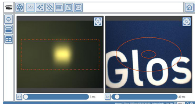
Aesthetix ® interactive measurements displays a live view from both cameras, ensuring perfect positioning and alignment on all surfaces.
