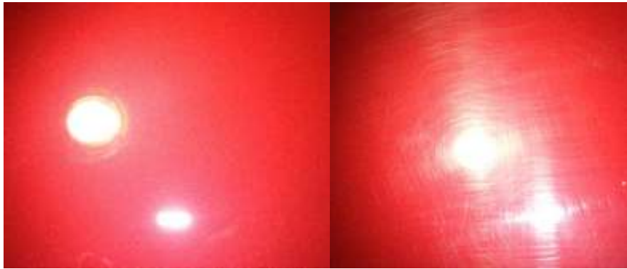
Reflected light sources in surfaces with medium and high haze values.
