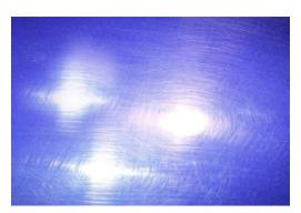
Haze is an important measure for highly polished metals and is often associated with polishing marks and machining direction.
