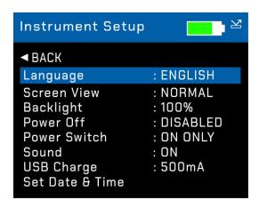
The Instrument Setup screen is used to configure the instruments basic operating environment to the user's preference. Press the <a href="Up / Down">Up / Down</a> buttons to navigate through the options, press the <a href="Enter">Enter</a> button to select the option required.
