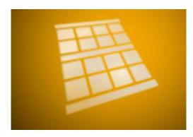
When viewing the reflection of a strong light source in a surface with high haze the image "blooms" and has a bright halo around it.
